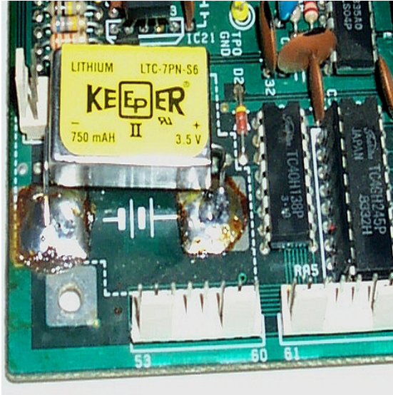
Figure 15 - New battery shown installed
