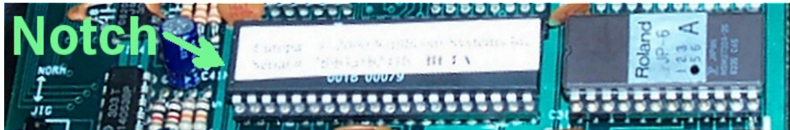
Figure 13 – Europa chip shown installed – Notched end to the LEFT!
