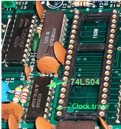
Figure 9 – Clock line “trace to cut” illustration
