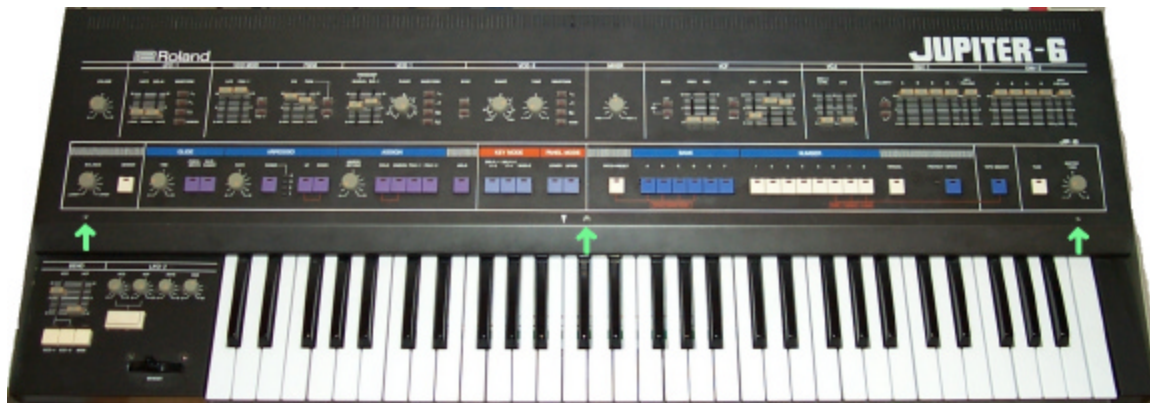
Figure 2 – JP-6 front panel screw locations
